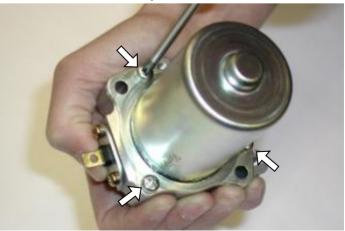
REMOVE DRUM FROM STARTER **KEEPING ROTOR IN ITS SEAT** (BE SURE TO HOLD THE ROTOR ON ITS TOOTHED SIDE TO PREVENT BRUSHES THE BRUSHES MAY SPRING OUT FROM FALLING OUT FROM THEIR SEAT) FROMTHEIR SEATS.
