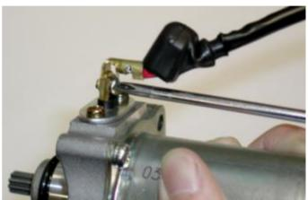
SECURE THE WIRE TO THE STARTER BY MEANS OF A PLASTIC CLAMP
